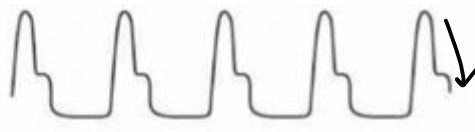
F Waterhammer (collapsing) pulse
